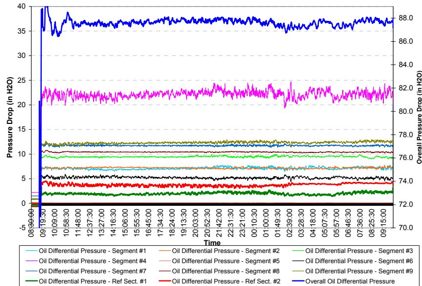
Figure A2 - Pressure Drops in Test 1
